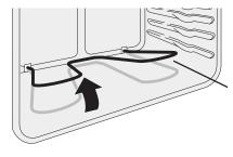
On models with visible bake element only; lower bake element may be raised from the front 4-5 inches to clean oven bottom.
